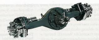
tractors. The tandem version is more than 60 pounds lighter than existing D170 series tandem axles, and it is available in a broad range of gear ratios, from 3.07 to 6.14, to serve a variety of needs.
