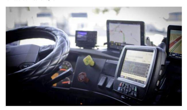
racking hours of service compliance is just a fraction of what most ELD systems can do. Some of the simplest, most inexpensive systems – often a smartphone app paired with an engine control module (ECM) connection device – come with web-based, back-office unit tracking software and dispatch tools. Others have more robust back-end programs.
