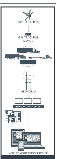
Rich data systems collect and transmit GPS positioning — latitude, longitude, state, city, and even the street name — for every trailer in your fleet, every ten minutes. Your rich data system should allow you to see which trailers are in motion, which are stopped, which are being powered by the tractor, and when ones have their doors open. Plus they provide real-time events like door status, cargo status and tractor power on/off. That's fleet visibility.
