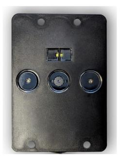
Spireon developed a new FleetLocate Cargo Sensor with IntelliScan sensing technology. The new sensor provides a new level of accuracy in visualizing cargo load status, the company says.
