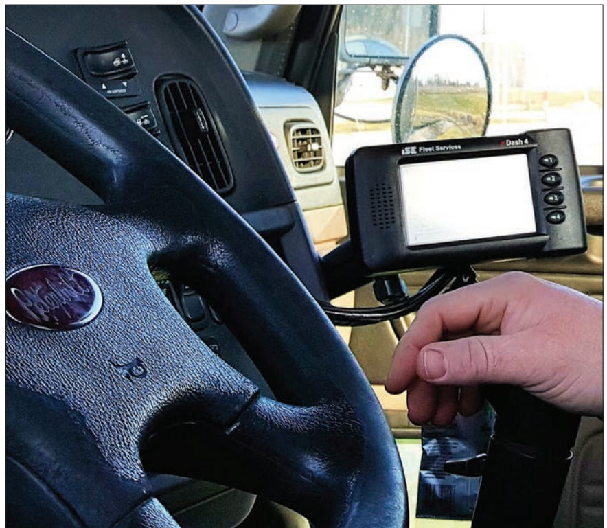
ISE Fleet Services' eFleetSuite baseline compliance device is a dedicated unit with its own cellular data connection but without a lot of extra functionality beyond logs.
