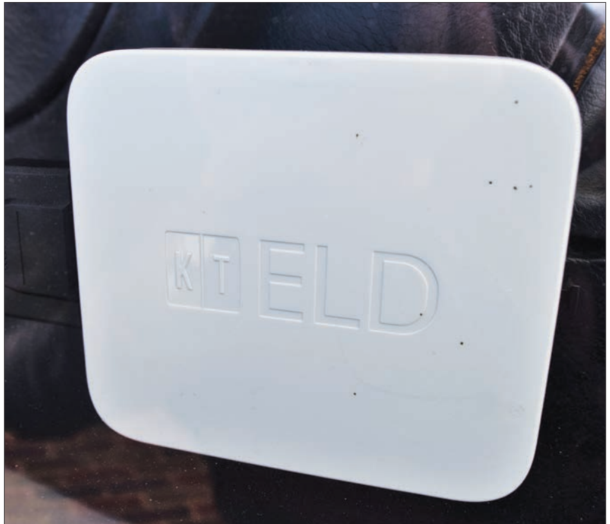
The KeepTruckin BYOD-style ELD "black box" connects to the ECM via cable and plugin. KeepTruckin recommends users mount the device in the dash to maintain a clear GPS connection. The device pairs with the KT app on a smartphone or tablet via Bluetooth connection.
