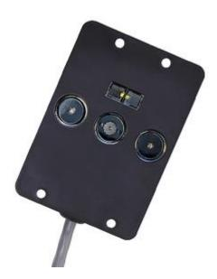
Spireon's new FleetLocate Cargo Sensor with IntelliScan is designed to resolve these issues by combining multiple sensors within a single device, and adding processing power to the sensors themselves. IntelliScan uses lasers for time-of-flight measurement, eliminating problems associated with cargo type and proximity. Laser technology is reliable and widely used in other industries, such as for pre-crash sensors in automobiles, where it detects pedestrians or other objects in the vehicle's way.
