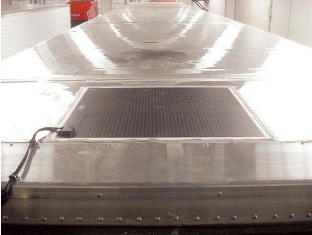
*Holland Enterprises uses solar panels on its trailers to supply power to its transport refrigeration units. Holland Enterprises Inc.*
