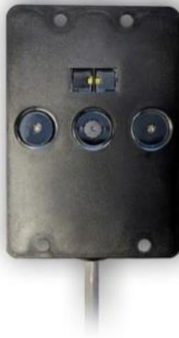
Spireon's new sensor is designed to resolve ultrasonic detection issues by combining multiple sensors within a single device, and adding sophisticated processing power to the sensors themselves.
